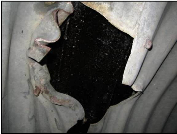
View inside hole in pipe wall. Appears to be another layer of metal material within the hole.
